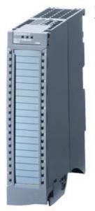
SIMATIC S7-1500, Analog input module AI 8xU/I HS, 16 bit resolution, accuracy 0.3% 8 channels in groups of 8, "Common mode voltage 10 V; diagnostics; Hardware interrupts 8 channels in 0.0625 ms oversampling incl. infeed element, Shield bracket and shield terminal
